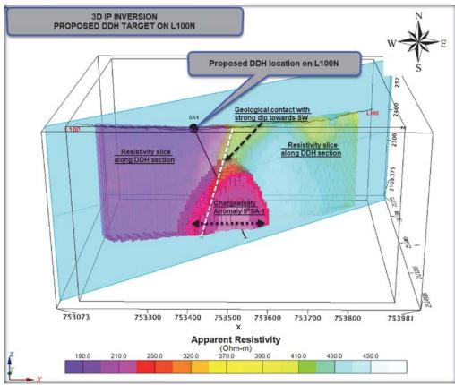
Interpretative 2D Cross Section of the IP chargeability anomaly (IPSA-1) superimposed over a resistivity slice along L100N, Oblique section view looking north (Simard, REPC\_276. Dec. 2017).
